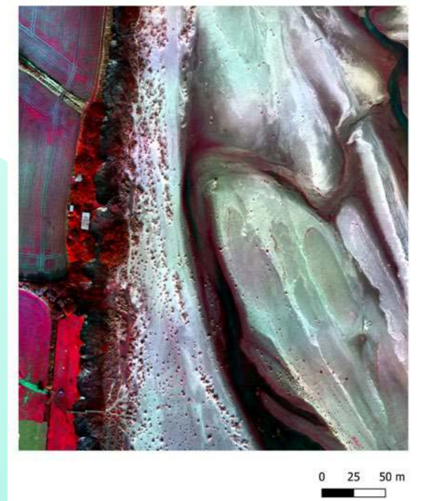
Figure 5: Multispectral imagery colour composite image. Bright red colours show healthy vegetation, black corresponds to water, green/grey colours are siltier sediment and white shows sand
