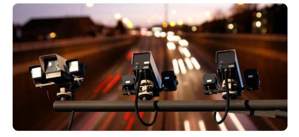
To avoid data protection concerns, only tractor unit registrations will be identified, no persons or other road users; the on-device data processing capability ensures that no video streaming will be required, reducing networking demands to suit 3G/4G capacity. It is important to note that such technology can be extended for dangerous goods placards, trailer numbers, vehicle length or size, to further improve data integration.
