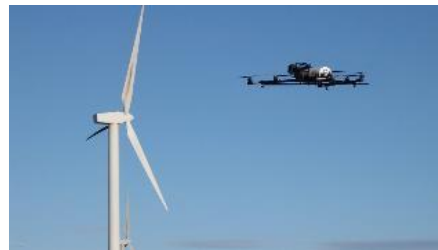
UAV blade inspections are being used
