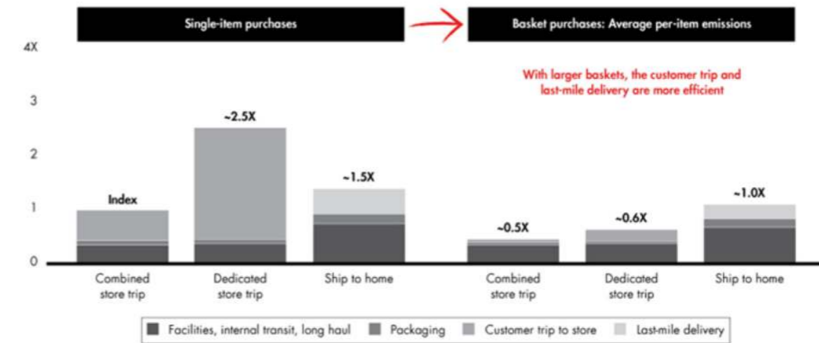
Figure 4: Lower carbon emissions from cluster purchases. source Bain & Co Emissions comparison across fulfillment channels (measured in carbon equivalents and indexed)
